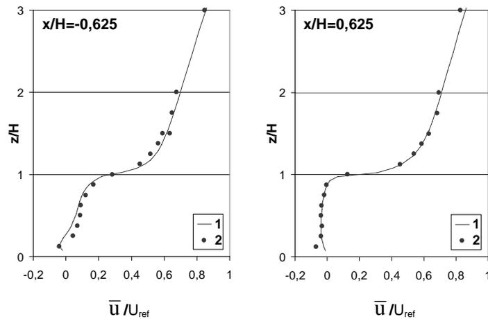
Figure 6. Comparison of the profile of the u velocity component observed in the wind tunnel with predictions at  $x/H=-0.625$  and  $x/H=0.625$  at  $y/H=0$  (- denotes upstream the cube centre). Numbers correspond to: 1 - model data; 2 - experimental data.
