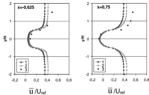
Figure 4. Comparison of the horizontal plots for  $u$  velocity component observed in the wind tunnel with predictions at  $x/H=-0.625$  and  $x/H=0.75$  at  $y/H=0$  (- denotes upstream the cube centre). Numbers correspond to: 1 - Case 1; 2 - Case 2; 3 - experimental data.
